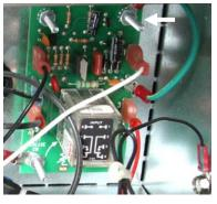
The time-delay relay board is shown in place above. The left photo shows the current placement of the mounting stud. The right photo shows the original grounding to a board mounting stud. Replacement of the board in either style grounding requires the ground wire terminal to be sandwiched between two nuts on the stud.
